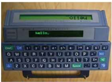
Fig. 7 A lightwriter used as a text to speech communication aid by people with speech loss
