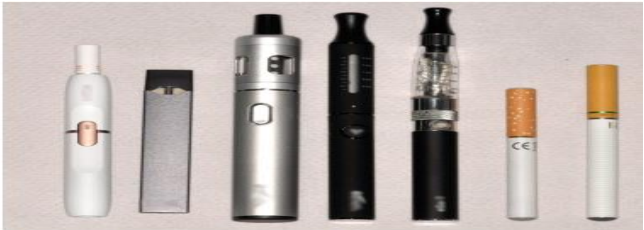
Figure 1. E-cigarette and heated tobacco devices in a range of designs. From right, two early devices that resemble a tobacco cigarette, so called 'cigalikes'; three 'tank' device which are refillable with e-liquids and rechargeable; a much smaller device that resembles an USB drive and uses nicotine salt technology; finally, a heated tobacco product with the tobacco stick in place.
